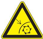
This symbol means that the guards must remain in place while the engine/motor on the machine is running because death or personal injury may result.
