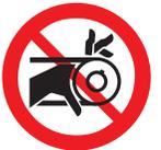
This symbol means do not insert fingers/digits under any edge of the belt cover while the engine/motor on the machine is running because personal injury and loss of fingers/digits may result. (Black pictogram with red "No" symbol outline)
