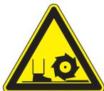
This symbol means that there are moving parts and if feet/fingers/digits are inserted under any edge of the cutter/grinder/saw cover while the engine/motor on the machine is running that personal injury and loss of foot/fingers/digits may result.
