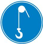
This symbol denotes the lifting point and means that if lifting of this equipment is necessary use a lifting device that is designed to accommodate or exceed the weight of this machine. Check the Operator's manual for specifications. Using a device that is not designed to accommodate or exceed the weight of this machine could result in damage to the machine and personal injury. Do not lift equipment over people because death or serious injury could result. (Blue background with white pictogram.)
