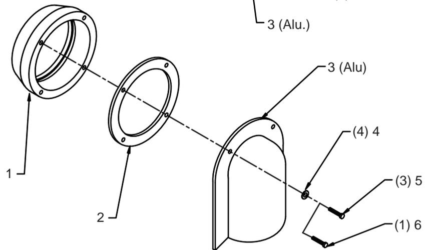
**PARTS LISTING - ILLUSTRATION #7 : 50mm INLET ASSEMBLY**
