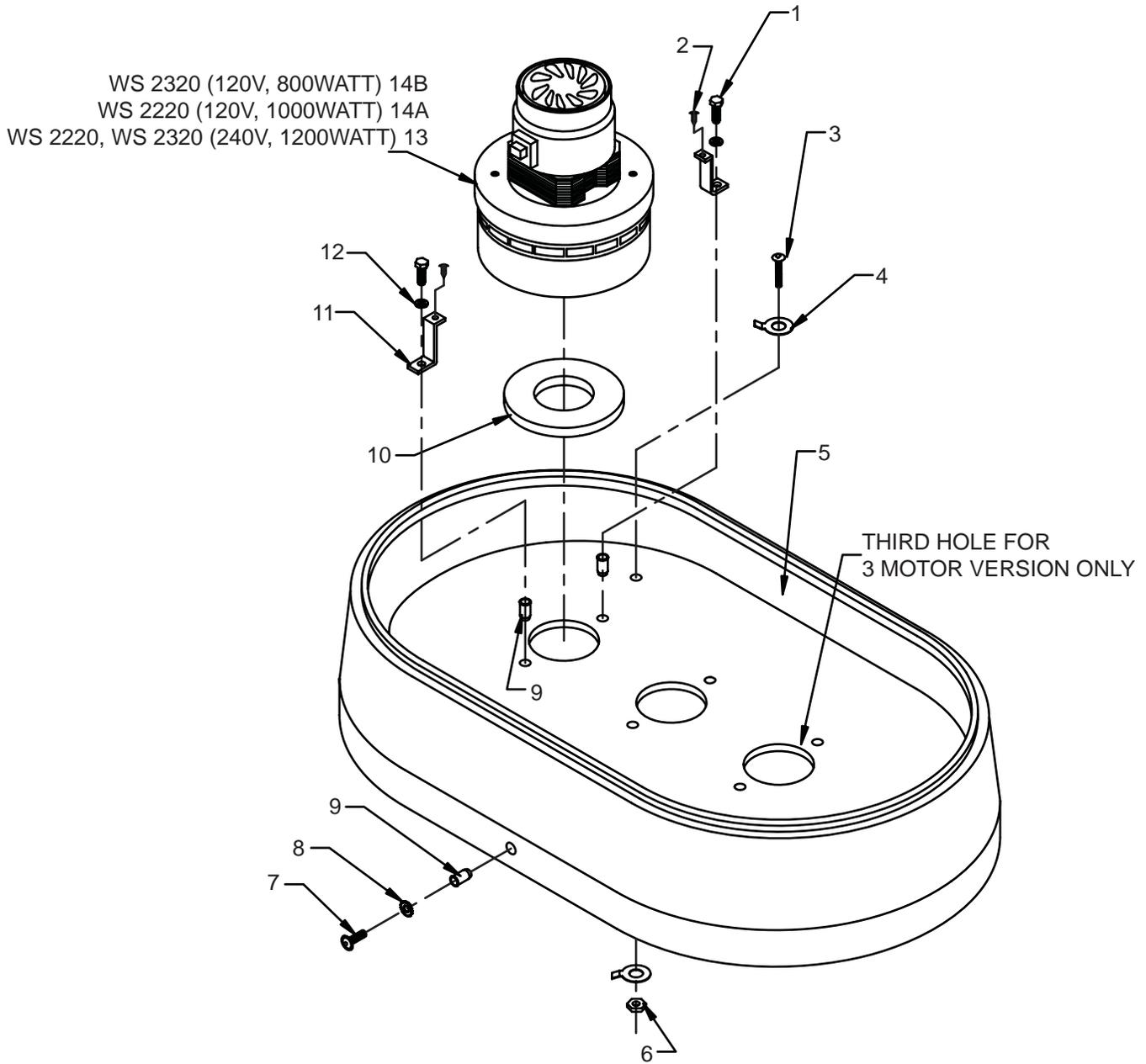
**PARTS LISTING - ILLUSTRATION #2 : WS2220 120V, 240V MOTOR ASSEMBLY**
