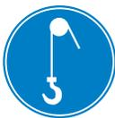
This symbol denotes the lifting point and means that if lifting of this equipment is necessary use a lifting device that is designed to accommodate or exceed the weight of this machine. Check the Operator's manual for specifications. Using a device that is not designed to accommodate or exceed the weight of this machine could result in damage to the machine and personal injury. Do not lift equipment over people because death or serious injury could result.
