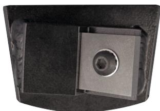
**MAGNA-BLADE** Magna-Blades use carbide tipped blocks to strip away coatings and clean floors without grinding into the concrete. The replaceable multisided tungsten carbide can be rotated for maximum use.
