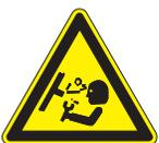
This symbol means hazardous pressures are present. Caution should be exercised to prevent personal injury or damage to equipment. Face, eye and head protection should be used.
