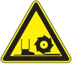
This symbol means that there are moving parts and if feet/fingers/digits are inserted under any edge of the cutter/grinder/saw cover while the engine/motor on the machine is running that personal injury and loss of foot/fingers/digits may result.
